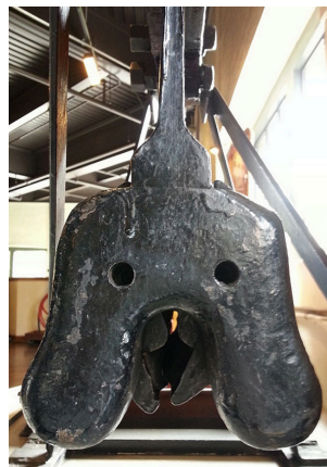
Grip (left) below the street, without the cable Gripman (right) in the car, pulling the grip
